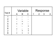
This is the most simple case. Can add more inputs and outputs. Do not have to test every combination.
